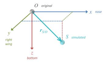
Figure 2.14: Simulated CG location axis convention.
