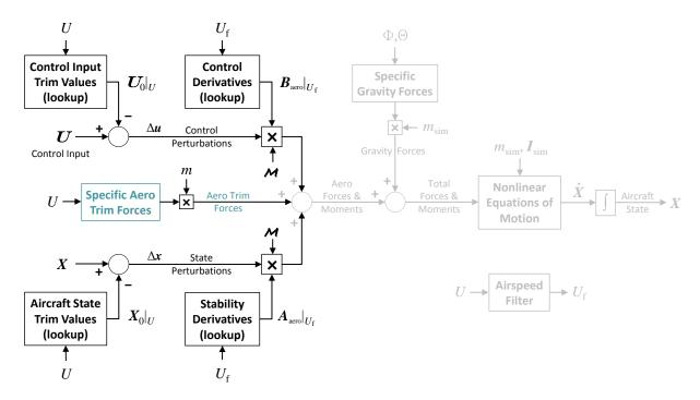
Figure 2.5: Model stitching simulation architecture – aero trim forces.
