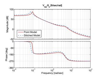
Figure 3.22: Case 2: true airspeed response to elevator input comparison.
