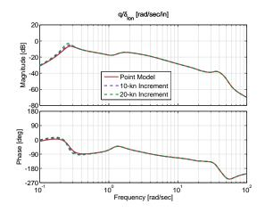
Figure 4.25: Pitch rate response to longitudinal cyclic input comparison for forward-flight trim data of 10- and 20-kn spacing, 80 kn.
