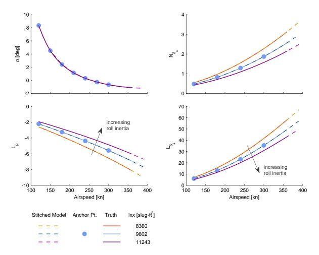
Figure 3.6: Verification of off-nominal inertia extrapolation, roll inertia  $I_{xx}$ .
