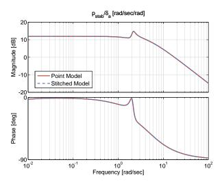
Figure 3.14: Case 1: roll rate response to aileron input comparison.
