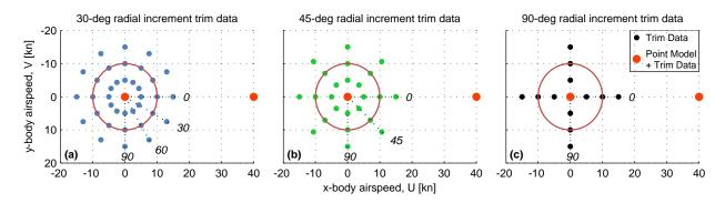
Figure 4.17: Trim data points at 30-, 45-, and 90-deg radial increments, with 10-kn magnitude indicated, and point models at hover and 40 kn.
