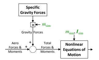
Figure 2.13: Simulation values of mass and inertia.
