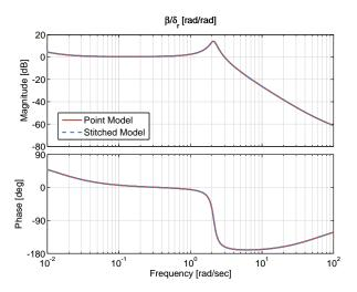
Figure 3.17: Case 1: sideslip response to rudder input comparison.
