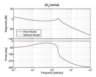
Figure 3.15: Case 1: sideslip response to aileron input comparison.
