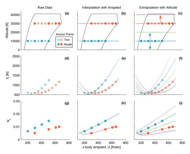
Figure 3.3: Spline-fit data and air density-ratio extrapolation to cover entire flight envelope.
