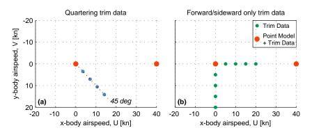
Figure 4.12: Quartering and pure forward/sideward flight trim data points at 5-kn airspeed  $V_{\text{tot}}$  increments, and point models at hover and 40 kn.
