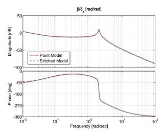
Figure 3.26: Case 2: sideslip response to aileron input comparison.
