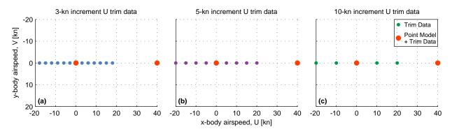
Figure 4.2: Forward/rearward flight trim data points at 3-, 5-, and 10-kn x-body airspeed U increments, and point models at hover and 40 kn.
