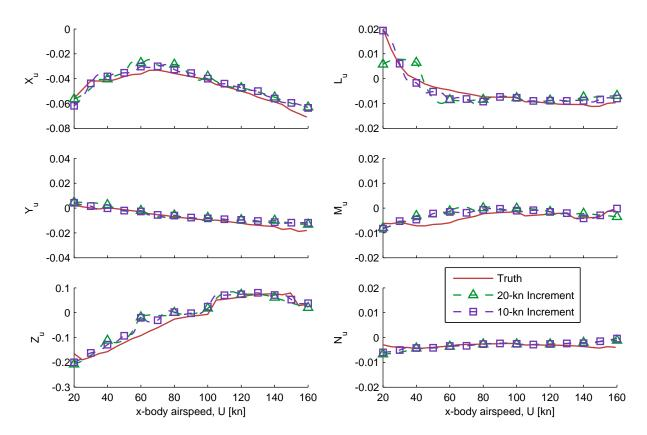
Figure 4.21: Implicit u-speed derivative values due to forward-flight trim data of 10- and 20-kn spacing.
