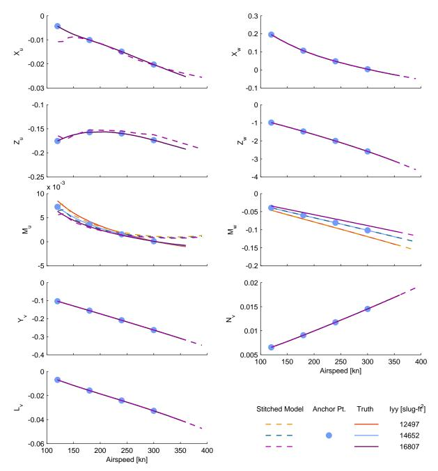
Figure B.7: Verification of off-nominal pitch inertia extrapolation, CJ1 stitched model, stability derivatives.
