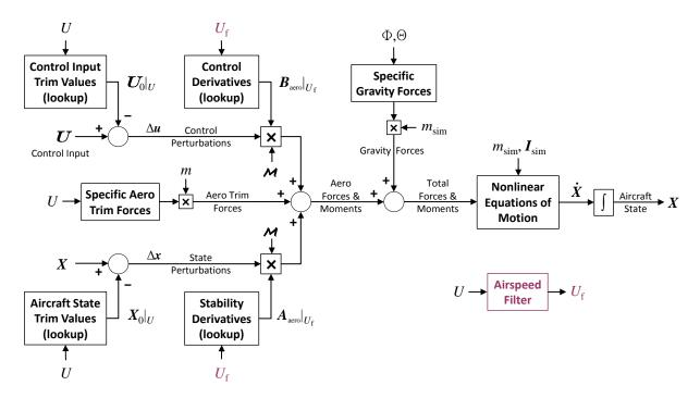
Figure 2.11: Model stitching simulation architecture – airspeed filter.
