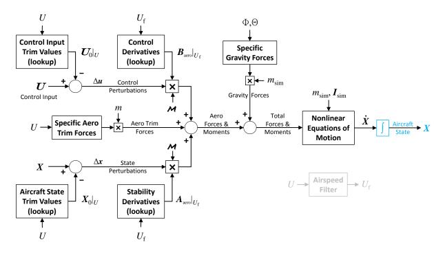
Figure 2.10: Model stitching simulation architecture – time integration.
