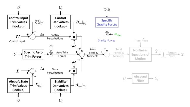
Figure 2.7: Model stitching simulation architecture – nonlinear gravitational forces.
