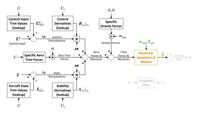
Figure 2.9: Model stitching simulation architecture – nonlinear equations of motion.
