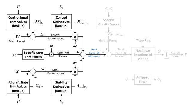
Figure 2.6: Model stitching simulation architecture – total aero forces and moments.
