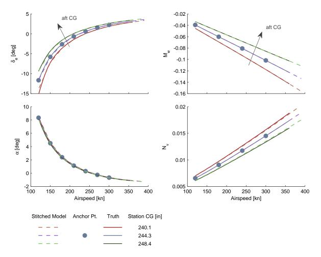
Figure 3.7: Verification of off-nominal CG extrapolation, fuselage station.
