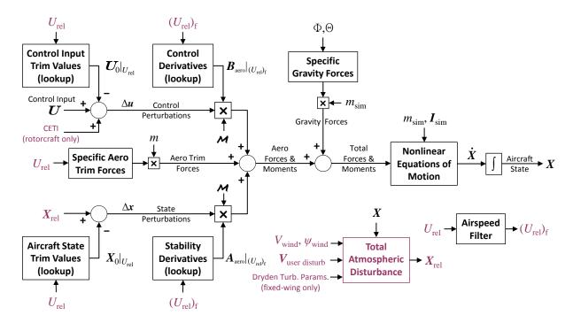
Figure 2.12: Model stitching simulation architecture – atmospheric disturbances.
