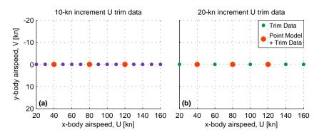
Figure 4.19: Forward-flight trim data points at 10- and 20-kn x-body airspeed U increments, and point models at 40, 80, and 120 kn.
