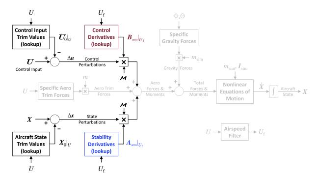
Figure 2.4: Model stitching simulation architecture – aero perturbation forces and moments.
