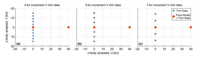
Figure 4.7: Sideward flight trim data points at 3-, 5-, and 7-kn y-body airspeed V increments, and point models at hover and 40 kn.
