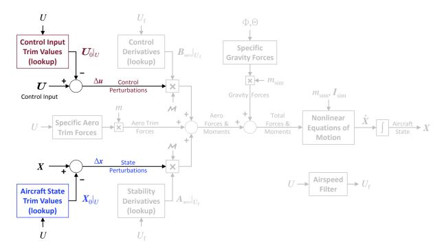
Figure 2.3: Model stitching simulation architecture – state and control perturbations.
