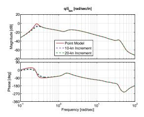
Figure 4.27: Pitch rate response to longitudinal cyclic input comparison for forward-flight trim data of 10- and 20-kn spacing, 120 kn.
