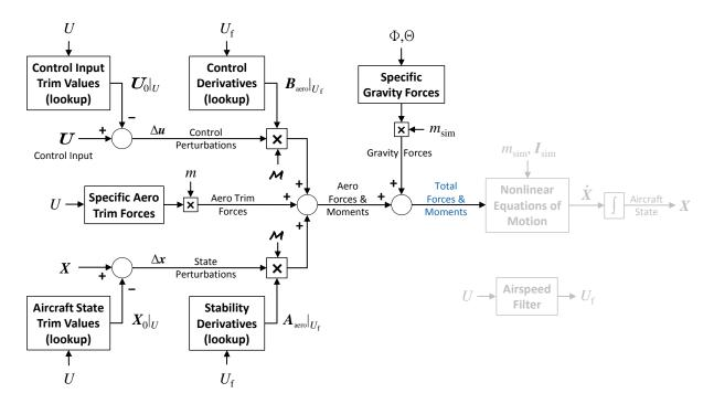
Figure 2.8: Model stitching simulation architecture – total forces and moments.
