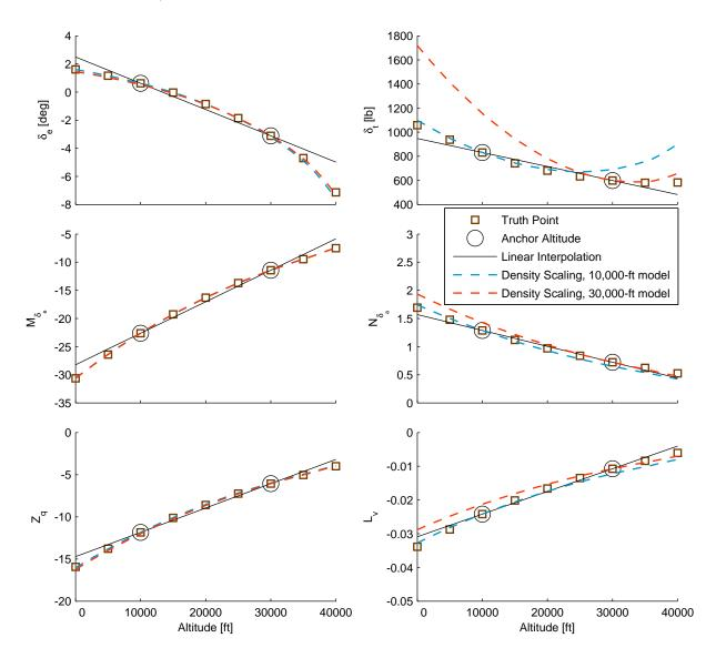
density-ratio scaling technique, as shown by the blue dashed lines for the 10,000-ft data, and by the orange dashed lines for the 30,000-ft data.
