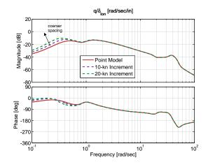
Figure 4.23: Pitch rate response to longitudinal cyclic input comparison for forward-flight trim data of 10- and 20-kn spacing, 40 kn.
