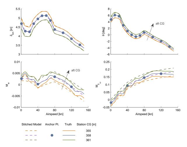
Figure 4.32: Verification of off-nominal CG extrapolation, fuselage station.
