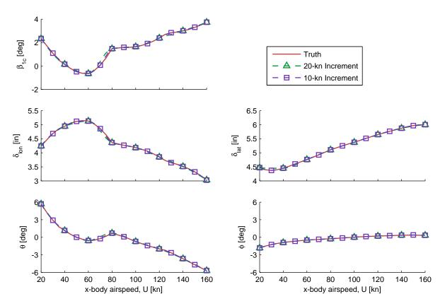
Figure 4.20: Spline-fit forward-flight trim values with 10- and 20-kn spacing.
