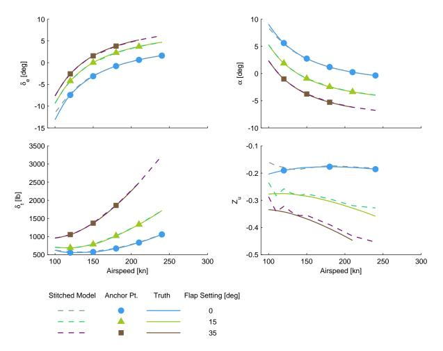
Figure 3.32: Alternate configuration verification, flap deflection.
