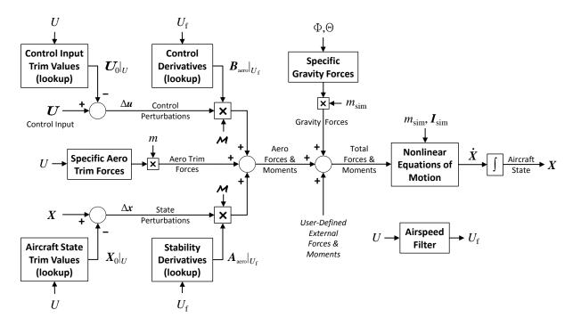
Figure 2.2: Model stitching simulation architecture – top level schematic.
