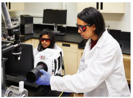
Mary Colleen Grace Meshach Ponraj, '20 MS Biomedical Engineering, operates the particle image velocimetry instrument while Hania Osman, '21 MS Biomedical Engineering, adjusts the camera for examination of the hemodynamic performance of a mechanical heart valve in vitro.
