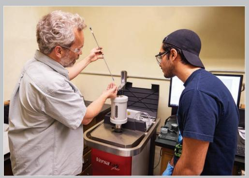
Dr. Brook demonstrates how to load and unload metallo-organic compounds from a physical property measurement system to Arshia Hamzehpour Savojbalaghi, '22 Biology (concentration in Systems Physiology). The system measures the magnetic properties of samples and how they change in different temperatures, from approximately 400K (344° Farenheit) to 50K (-369.4° Farenheit).
