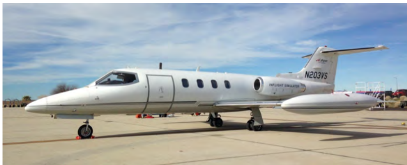
Figure 2. Calspan Variable Stability System Learjet LJ-25D.
