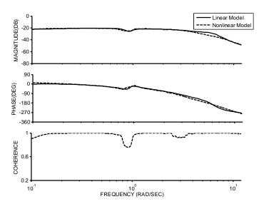
Figure 20.  $\phi/\delta_{lat}$  closed loop validation of nonlinear responses for the pilot handling control system.
