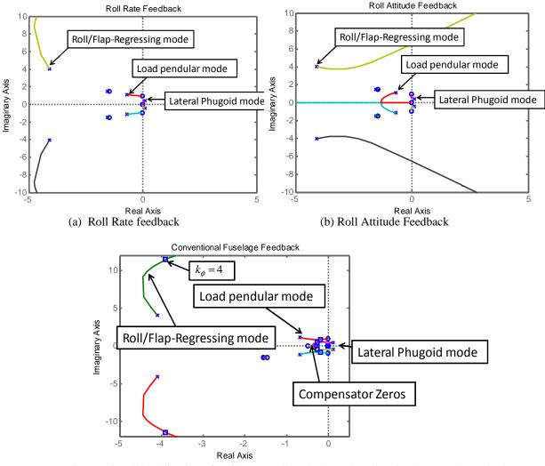
(c) Conventional Combination of Roll Rate, Roll Attitude, and Roll Attitude Integral Feedback
