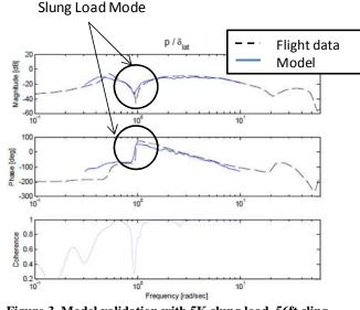
Figure 3. Model validation with 5K slung load, 56ft sling.  $$4^{-4}$$
