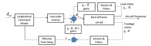
Figure 13. Longitudinal controller architecture.
