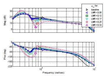
Figure 4. Roll attitude frequency response due to lateral cyclic for the 79ft sling with increasing LMR (Ref. 2).
