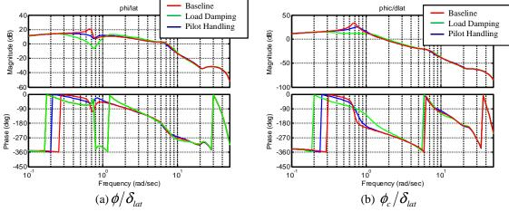
Figure 17. Closed loop bode plot overlays for three optimized control systems.
