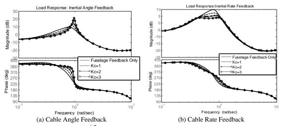
Figure 11. Load response  $\phi_c/\delta_{lat}$  bode plot for combined fuselage and cable angle/rate feedback.
