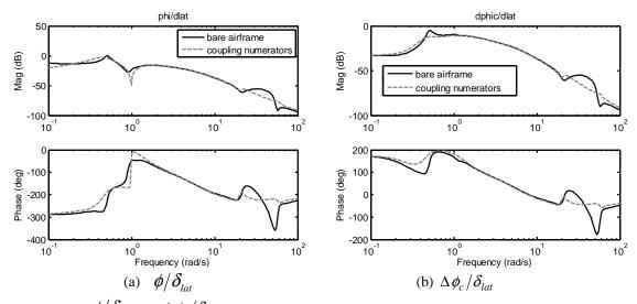
Figure 6.  $\phi/\delta_{lat}$  and  $\Delta\phi_c/\delta_{lat}$  with and without coupling numerator closure of the off-axis dynamics.
