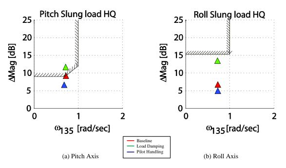
Figure 16. Slung load handling qualities specification for three optimized control systems.
