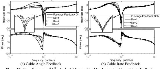
Figure 10. Aircraft response  $\phi/\delta_{lat}$  bode plot for combined fuselage and cable angle/rate feedback.
