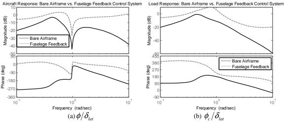
Figure 8: Bode plot comparison between bare airframe and fuselage feedback.
