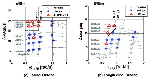
Figure 5. Slung load handling Qualities criteria (Ref. 2), where HQR>4 represents poor handling.
