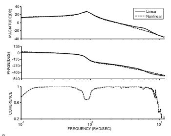
Figure 21.  $\phi_c/\delta_{lat}$  closed loop validation of nonlinear responses for the pilot handling control system.
