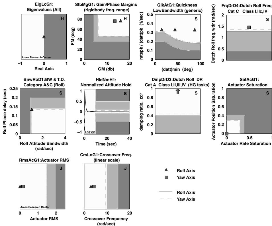
Fig. 5. Optimal Classical Design Characteristics
