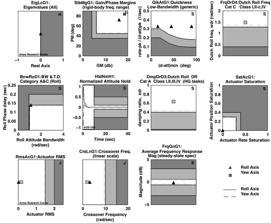
Fig. 10. Optimized LQR Control System Characteristics.
