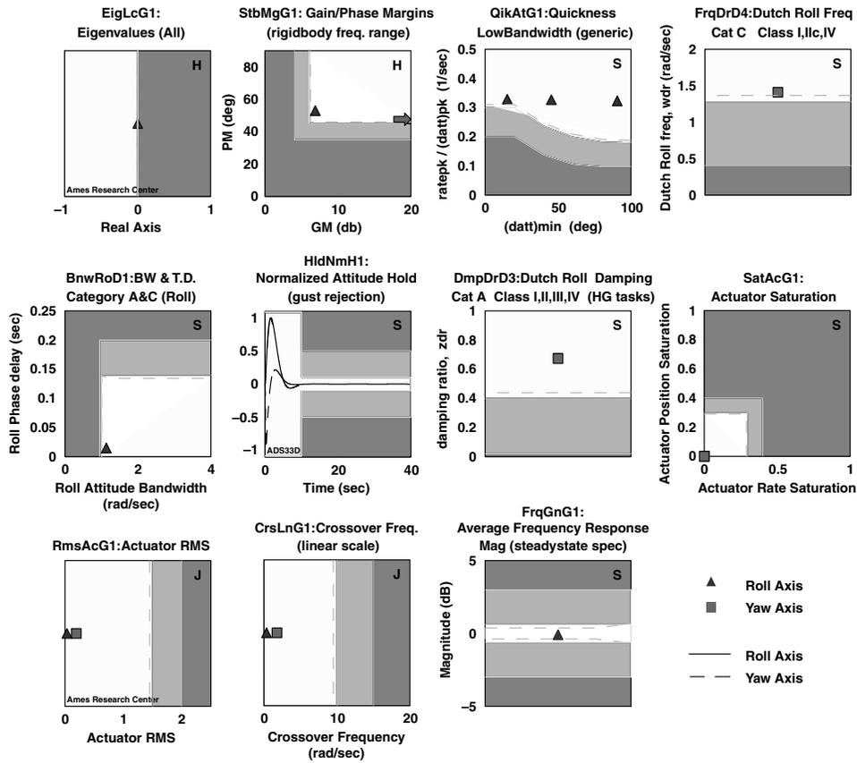
Fig. 14. Optimized Dynamic Inverse Control System Characteristics.
