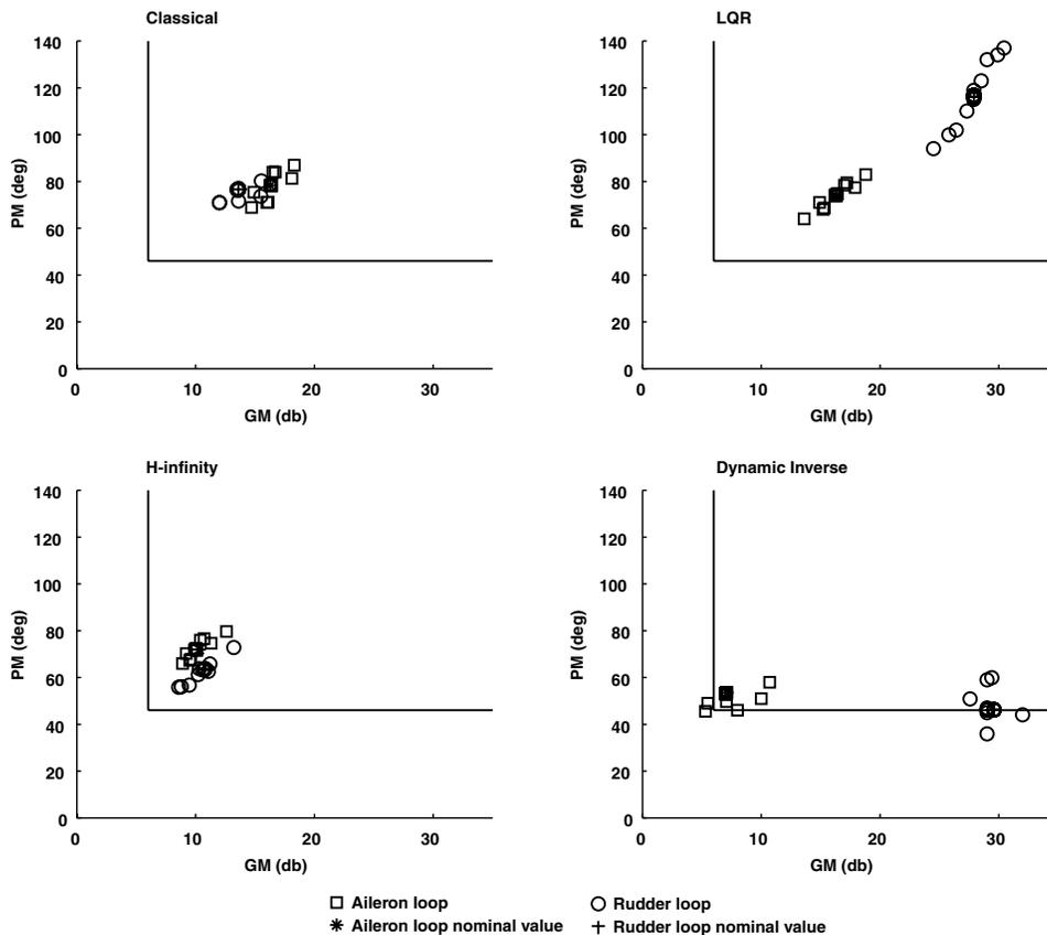
Fig. 19. Robustness Comparison for 20% Plant Variations.
