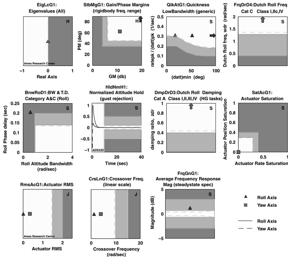
Fig. 16. Initial Design for H-infinity Control Law Design.
