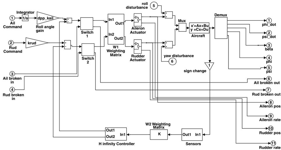
Fig. 15. H-infinity Control System Architecture.
