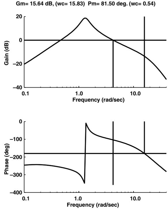
Fig. 6b. Rudder Broken-Loop Response (Optimized).
