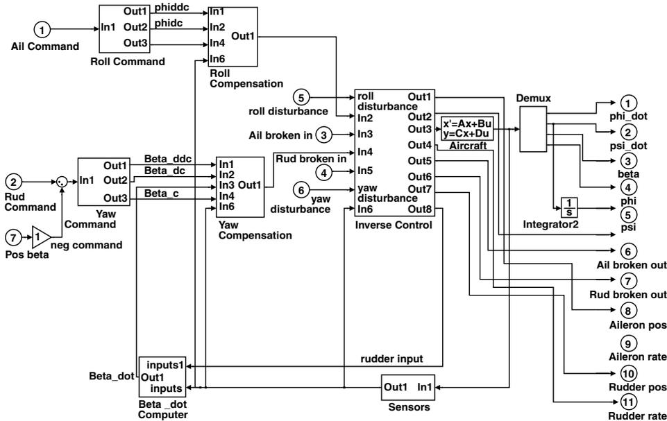
Fig. 11. Dynamic Inverse Control Architecture.
