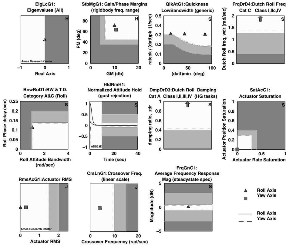
Fig. 18. Optimized H-infinity Control System Characteristics.
