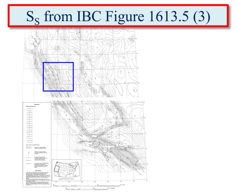
FIGURE 1613.5(3)—continued MAXIMUM CONSIDERED FAITHOUAKE GROUND MOTION FOR REGION 1 OF 0.2 SEC SPECTRAL RESPONSE ACCELERATION (5% OC ENTICAL DAMPINO), SITE CLASS B
