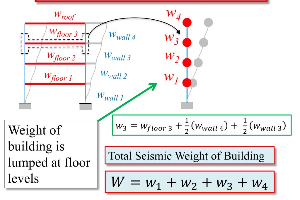
Equivalent Static Seismic Forces and Seismic Base Shear
