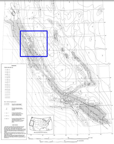
FIGURE 1613.5(4)—continued MAXIMUM CONSIDERED EARTHQUAKE GROUND MOTION FOR REGION 1 OF 1.0 SEC SPECTRAL RESPONSE ACCELERATION (5% OF CRTICAL DAMPING), SITE CLASS B
