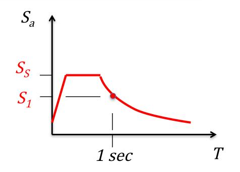
Acceleration at bedrock  $S_s$  and  $S_1$  from IBC Figures 1613.5 (3 and 4)
