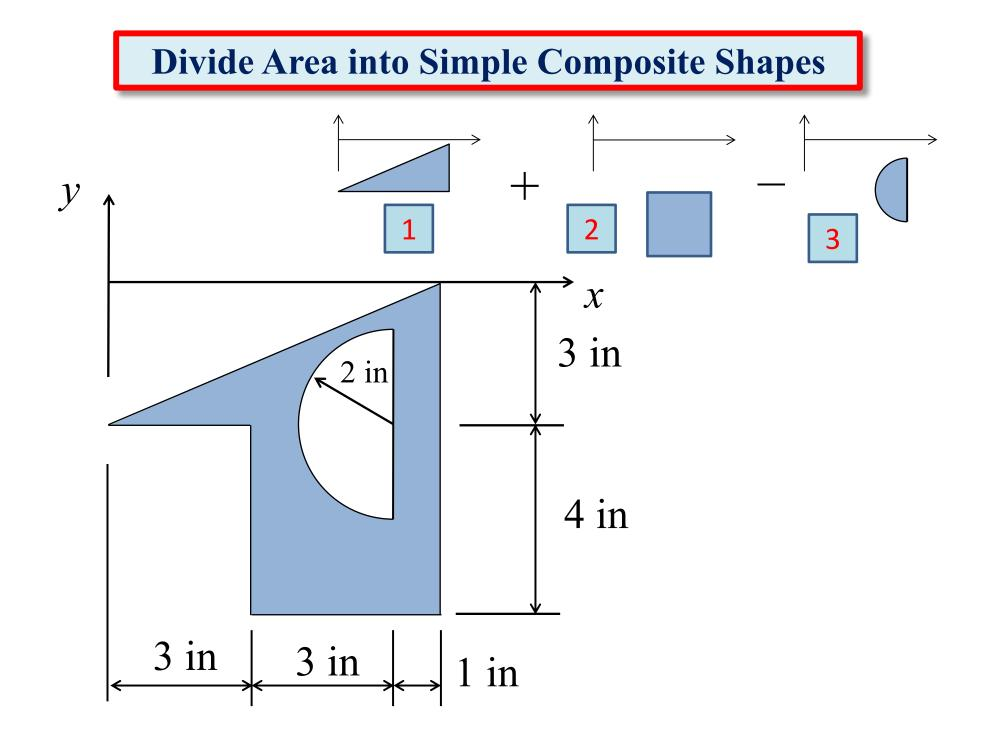
Find the Area, Location of Centroid, and the Centroidal Moment of Inertia of Each Shape
