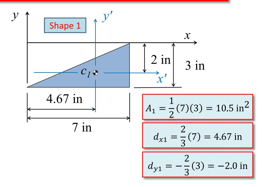
Find the Area, Location of Centroid, and the Centroidal Moment of Inertia of Each Shape
