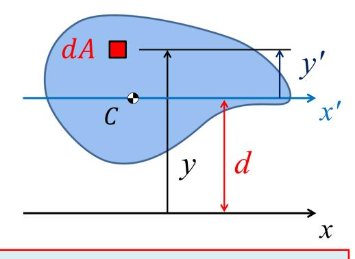
Consider an axis *x* 'that is parallel to the *x* axis and passes through the centroid of the area. The distance between the two parallel axes is *d*
