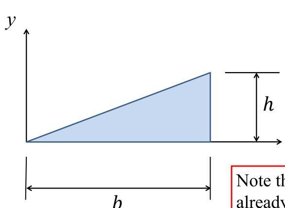
Find the Moment of Inertia of the of the shaded area about the *x* and *y* axes shown. Use the Parallel Axis Theorem.
