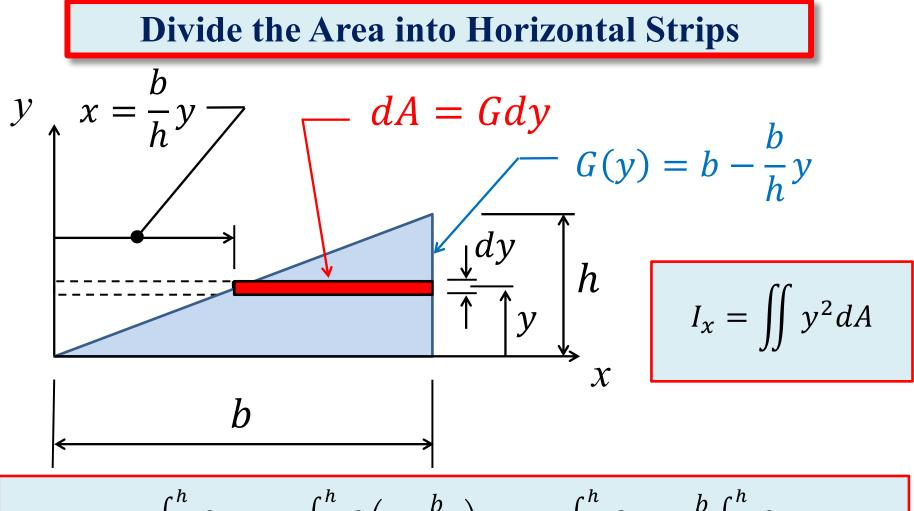
$$I_x = \int_0^n y^2 \, G \, dy = \int_0^n y^2 \left( b - \frac{b}{h} y \right) \, dy = b \int_0^n y^2 \, dx - \frac{b}{h} \int_0^n y^3 \, dx$$
