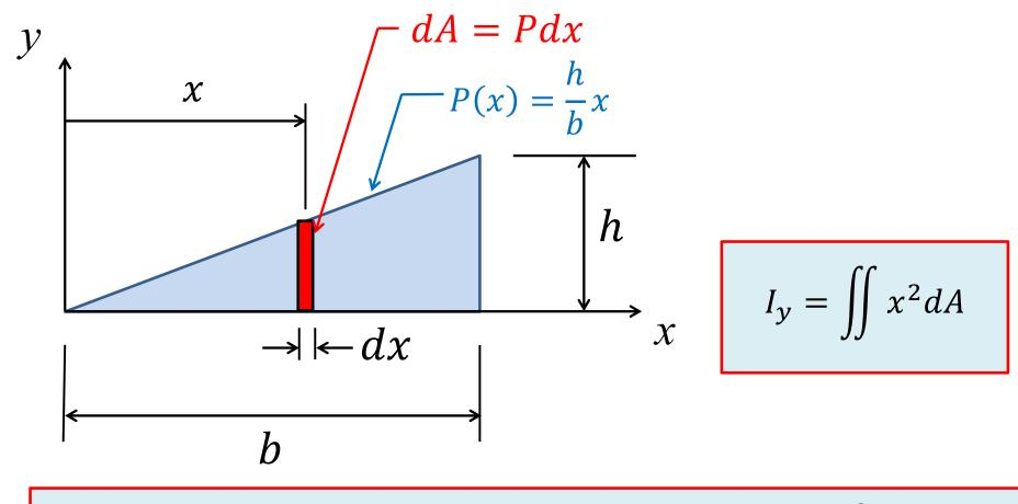
$$I_{y} = \int_{0}^{b} x^{2} P dx = \int_{0}^{b} x^{2} \left(\frac{h}{b}\right) x dx = \frac{h}{b} \int_{0}^{b} x^{3} dx = \frac{h}{b} \left[\frac{x^{4}}{4}\right]_{0}^{b} = \frac{1}{4} b^{3} h$$
