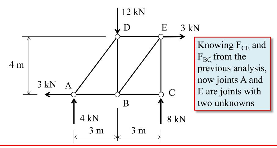
3. Draw a FBD of a truss joint adjacent to the joint analyzed in Step 2 that has no more than **two unknowns** (using the results from Step 2) use the **two equations of equilibrium** to find the two unknown truss member forces;
