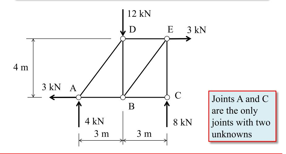
2. Draw a FBD of a truss joint that has no more than **two unknowns** and use the **two equations of equilibrium** to find the two unknown truss member forces;
