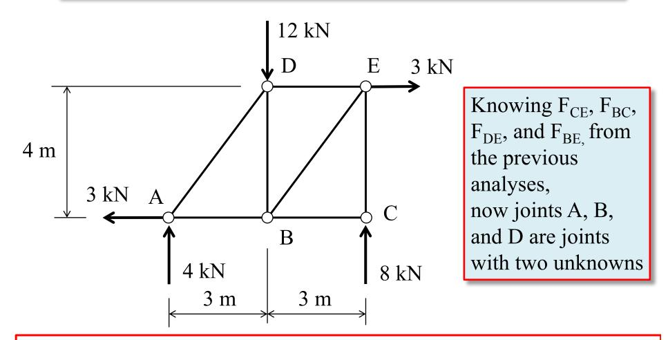
Repeat Step 3 until all truss member forces are found – a good check is if the last truss joint is in equilibrium then one has good confidence that the analysis is correct.
