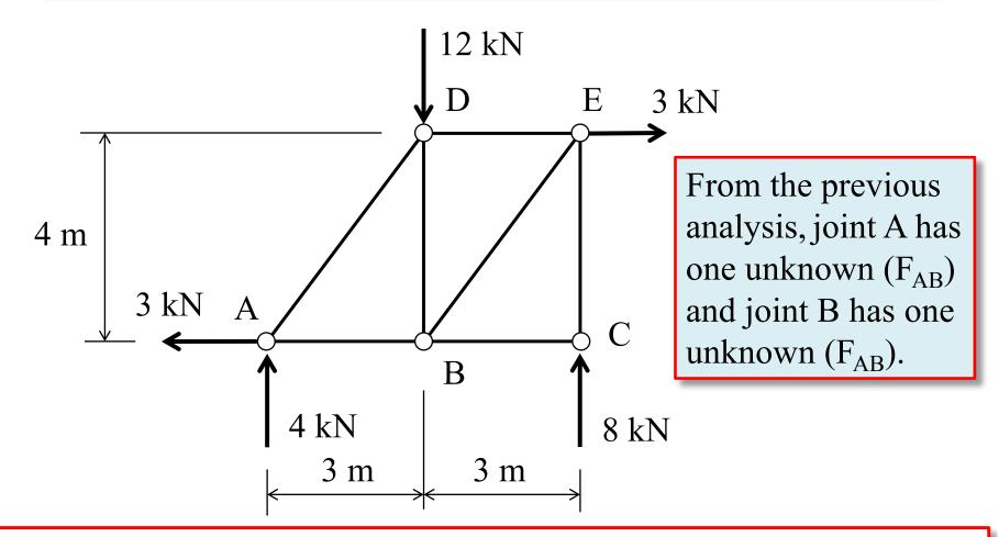
Repeat Step 3 until all truss member forces are found – a good check is if the last truss joint is in equilibrium then one has good confidence that the analysis is correct.
