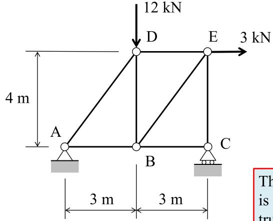
Consider the idealized truss structure with a pin support at A and a roller support at C. The truss is subjected to applied loads at D and E.
