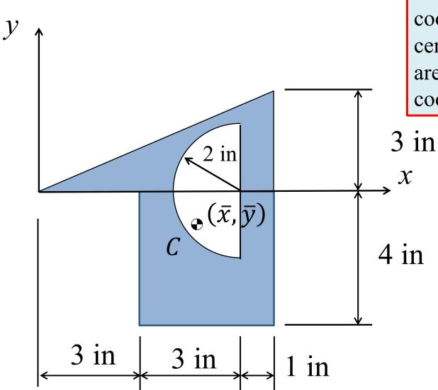
Find the *x* and *y* coordinates of the centroid of the shaded area with respect to the coordinate axes shown.
