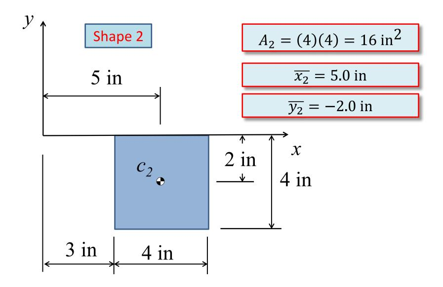
Find Area and Location of Centroid of Each Shape Relative to Reference Coordinate Axes
