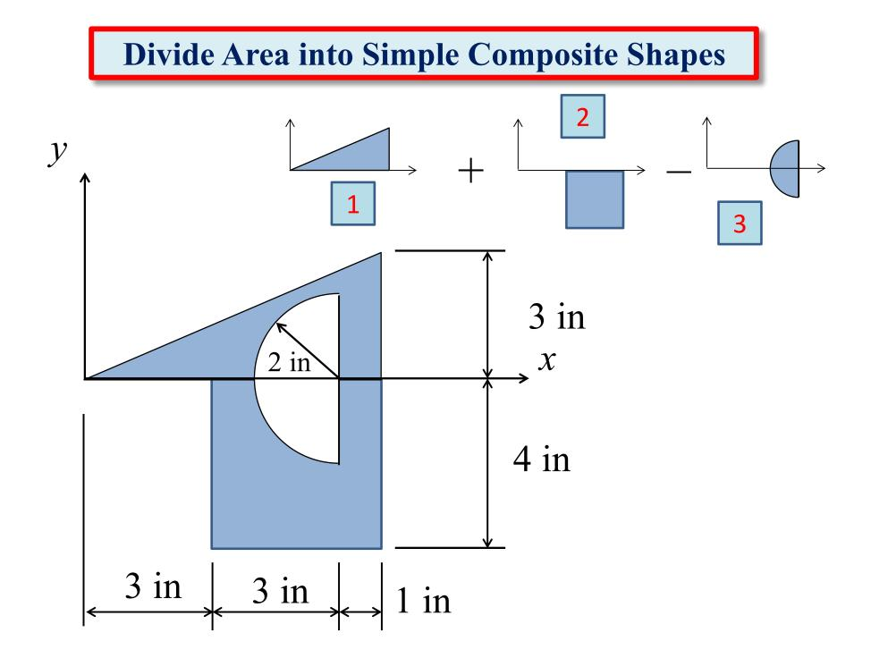
Find Area and Location of Centroid of Each Shape Relative to Reference Coordinate Axes
