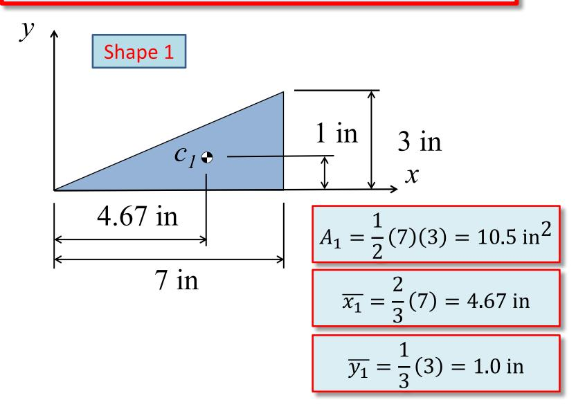
Find Area and Location of Centroid of Each Shape Relative to Reference Coordinate Axes
