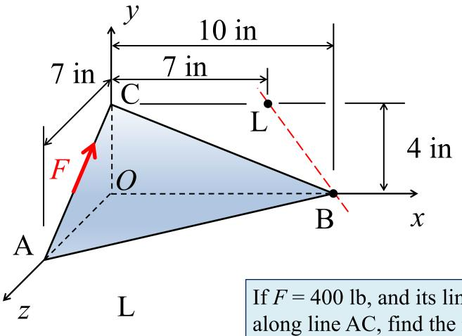
If F = 400 lb, and its line-of-action lies along line AC, find the moment of the force about the axis defined by line BL that lies in the *xy* plane.
