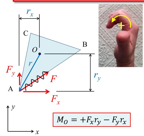
Calculate the moment of each component of *F* using the perpendicular distance from point *O*.
