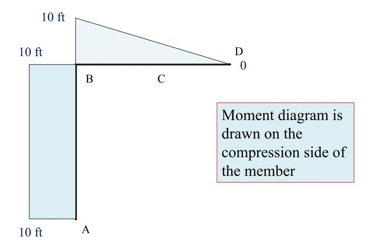
M<sub>Q</sub> Diagram for the Flexibility Coefficient Problem
