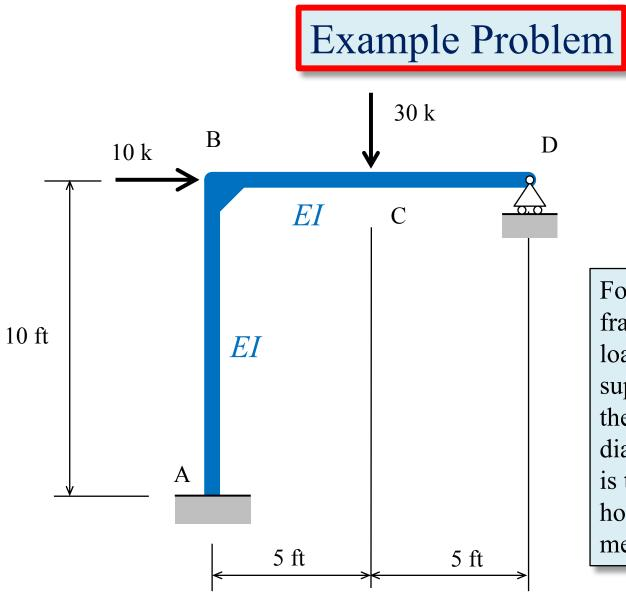
For the indeterminate frame subjected to the point loads shown, find the support reactions and draw the bending moment diagram for the frame. *EI* is the same for both the horizontal and vertical members.
