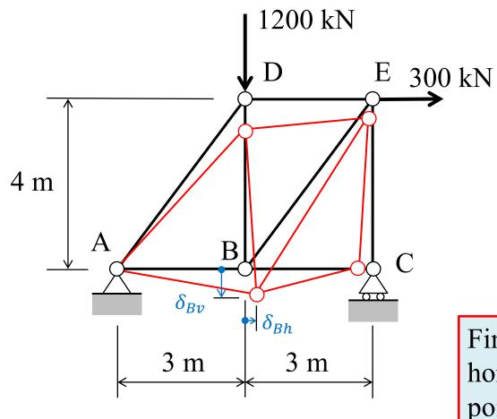
For all truss members use:  $A = 25 \text{ cm}^2$ E = 210 GPa Consider the idealized truss structure with a pin support at A and a roller support at C. The truss is subjected to applied loads at D and E.
