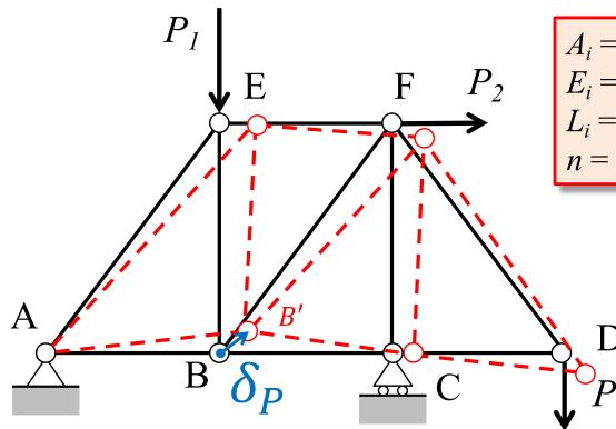
$A_i$  = Cross sectional area  $E_i$  = Modulus of Elasticity  $L_i$  = Length of truss member n = Total number of truss members
