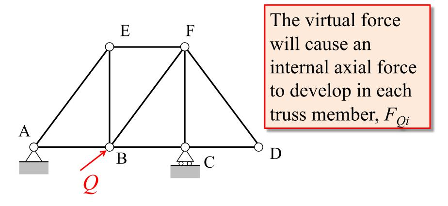
Apply a virtual force **in-line** with the real displacement  $\delta_P$
