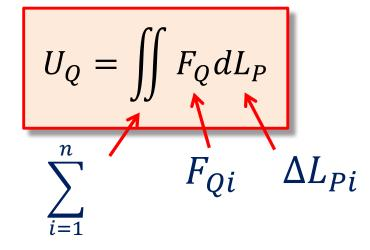
Virtual strain energy developed in an individual truss member *i*
