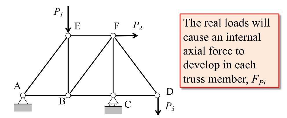
$A_i$  = Cross sectional area  $E_i$  = Modulus of Elasticity  $L_i$  = Length of truss member n = Total number of truss members The real loads cause an axial deformation of each truss member,  $\Delta L_{Pi} = \frac{F_{Pi}L_i}{A_i E_i}$
