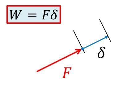
Work is done by a force acting through and in-line displacement
