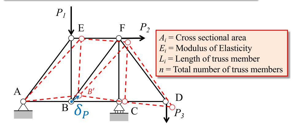
We want to find the deflection of joint B due to the applied loads
