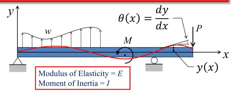
We seek y(x) and  $\theta(x)$  that describe the transverse deformation of the neutral axis and the slope of the tangent line to the neutral axis.
