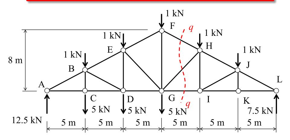
2. Make a cut through the members of the truss that are of interest. The cut must define two separate sections of the truss;
