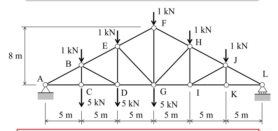
Consider the idealized truss structure with a pin support at A and a roller support at L. The truss is subjected to applied loads shown. Find the truss member forces FH, GH, and GI 1. Draw a Free Body Diagram (FBD) of the **entire truss** cut loose from its supports and find the **support reactions** using the equations of equilibrium (we will see that for some truss structures this step is not always necessary)
