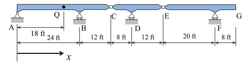
A beam is pin supported at point A and roller supported at points B, D, and F. The beam contains internal hinges at points C and E.
