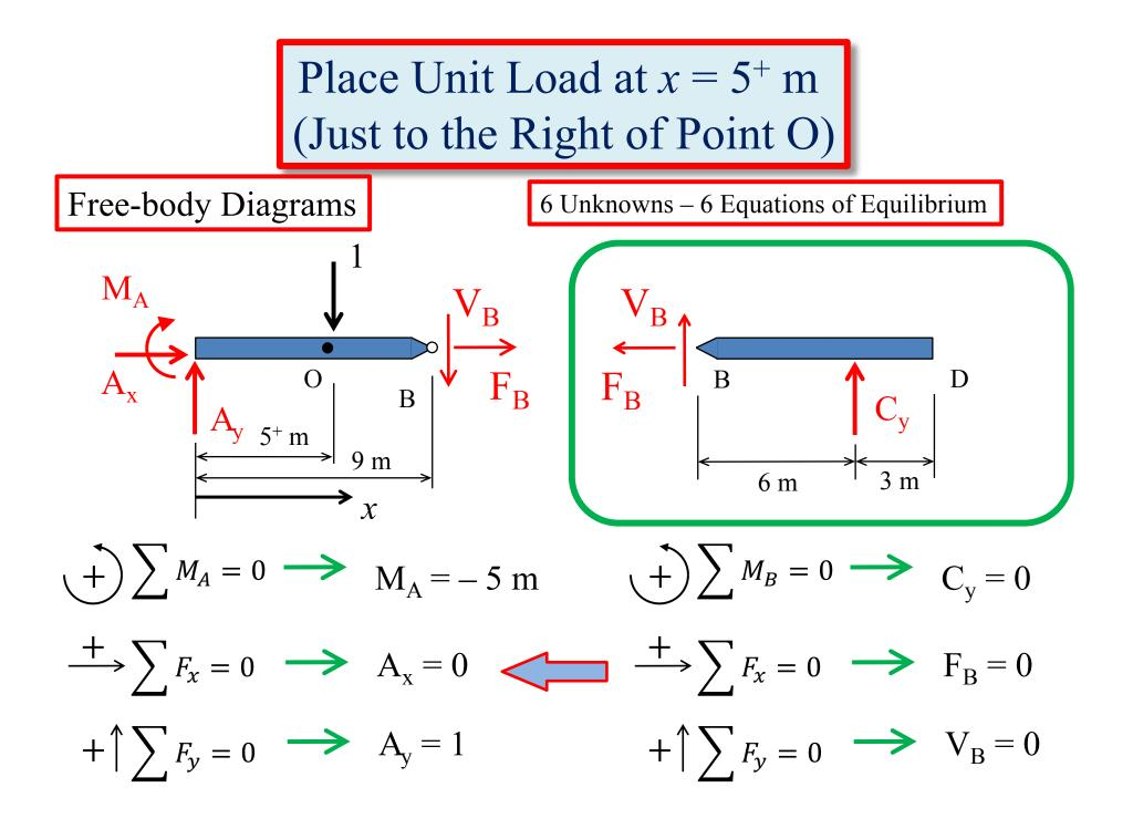
FBD of Segment OB for Unit Load at  $x = 5^+$  m (Just to the Right of Point O)
