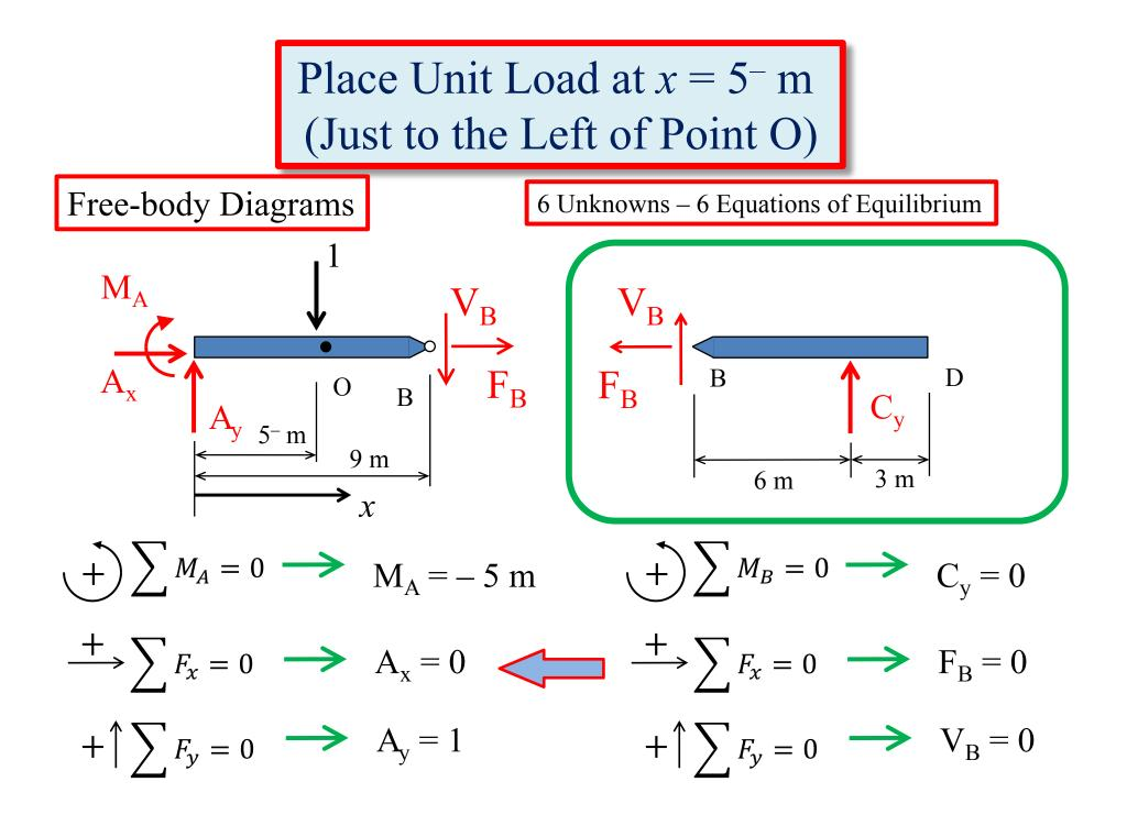
FBD of Segment OB for Unit Load at  $x = 5^{-}$  m (Just to the Left of Point O)
