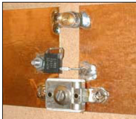
Figure 4 Resonance capacitor and damping resistor
