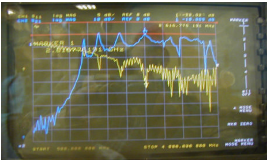
Picture 3: S_{11} and S_{21} measurements while tuning the waveguide
