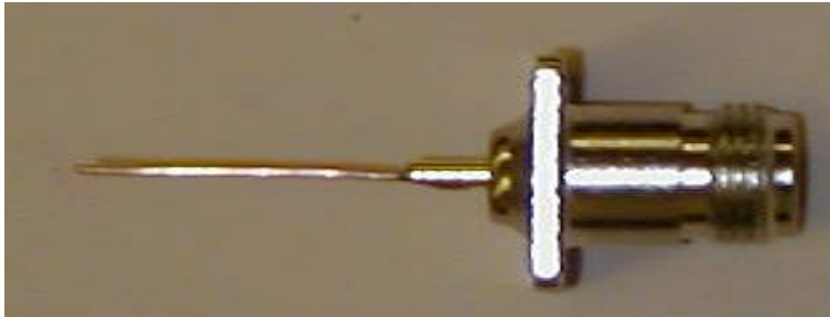
Picture 2: N-connector with a 1.18 inches of copper wire attached to it
