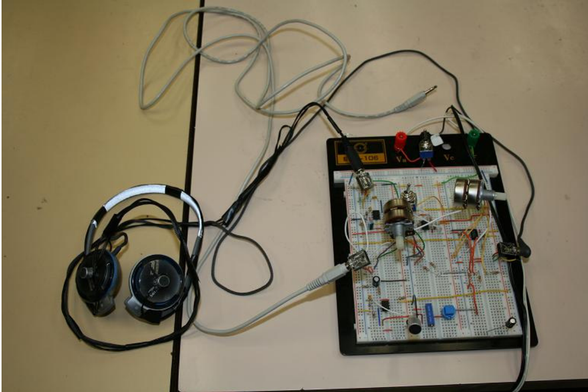
Picture 1. Communication System Breadboard Implementation
