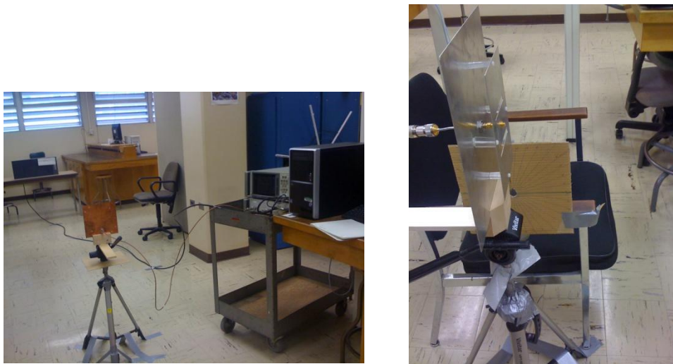
Figure 4 Setup of the radiation measurement with the transmitting antenna in the background.
