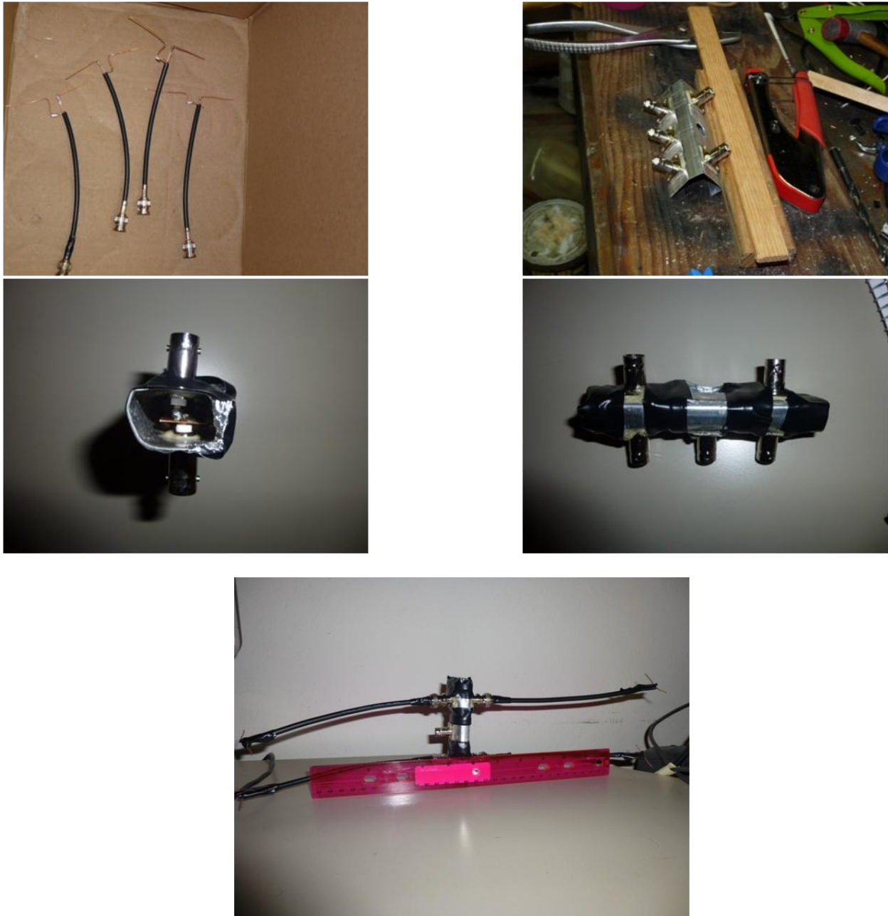
Figure 21: The Dipole Antennas after construction and before electrical tape was used to make the separation between the two quarter-wave wires smaller. Construction of the stripline power divider with a side view as well as a view of the center conductor. The completed 2 by 2 Dipole Antenna Array.
