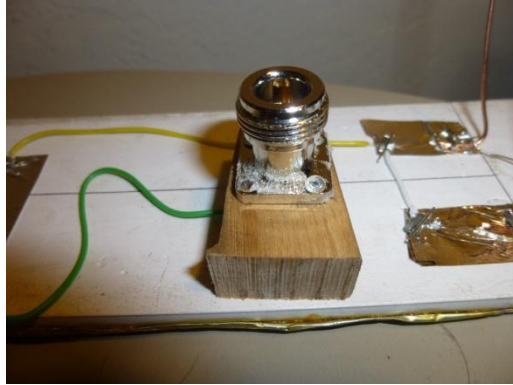
Figure 34: The N-type female connector on the 2 by 2 Monopole array that was not grounded.
