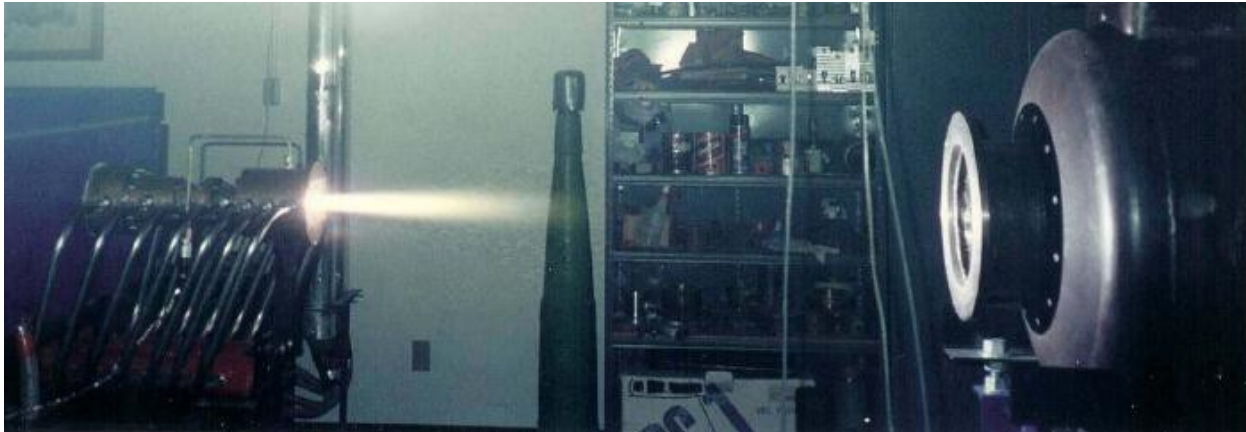
Fig.1.1: Arc jet at Aerodynamic Research Center of UT-Arlington: The picture above was taken several years ago where the arc jet is not directly connected to the test section chamber. [25]
