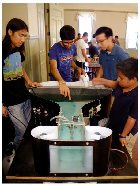
Figure 2: A 4<sup>th</sup>-grader observing the flow streamlines around a model airplane in a portable water tunnel.
