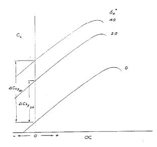
Figure 5.2. General Effect of Trailing Edge Devices on Lift Curve Slope [29]
