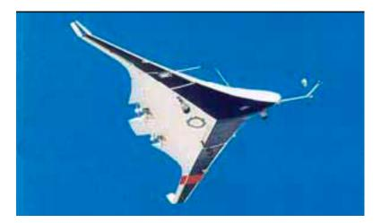
Figure 1.7. Remote Controlled 6% Model, BWB-17 [4]
