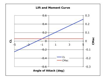
Figure 4.12. Wing Lift and Moment Curve (Linear Range)
