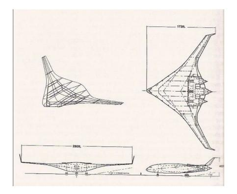
Figure 1.6. Three View Drawing of 800 Passenger BWB Design [5]
