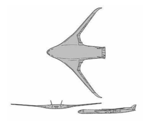
Figure 1.5. First Generation Blended Wing Body [4]
