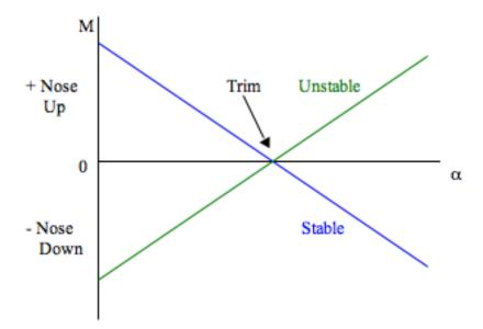
Figure 4.1. Aircraft Pitching Moment vs Angle of Attack
