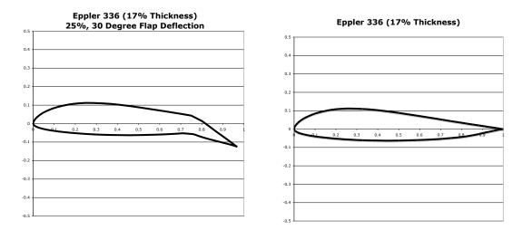
Figure 5.3. Effect on Camber of Reflexed Airfoil With Trailing Edge Flap
