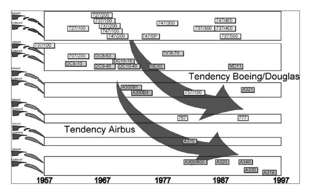
Figure 5.1. Design Evolution of Trailing Edge Devices [27]
