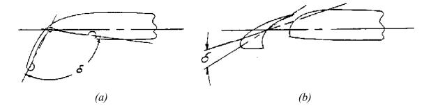
Figure 5.6. Geometry of (a) Krueger Flap and (b) Slat [29]
