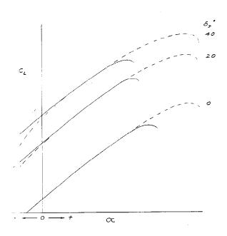
Figure 5.5. Effect of Leading Edge Devices
