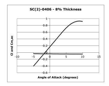
Figure 4.9. SC(2)-0406 Lift and Moment Curve ( $Re=1x10^8$ )
