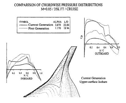
Figure 2.4. Pressure Distributions For Inboard and Outboard Airfoils [2]
