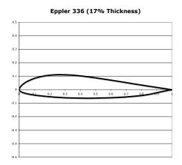
Figure 4.5. Eppler 336 Airfoil
