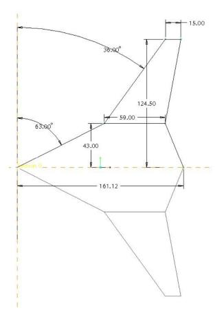
Figure 2.3. Approximate Wing Geometry
