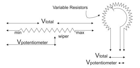
The output voltage in both scenarios varies according to the location of the sliding contact on the resistor. Ideally, distance would be perfectly proportional to the output voltage. Unfortunately, this is not the case due to the non linear characteristics of the resistive element and the additional load of the sliding contact.
