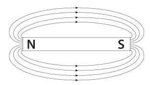
When the strong external force goes away the domains would relax and go random again unless a strong internal force (coercivity of the material) takes control while the strong external force is present. Internal mechanisms that develop coercivity are "anisotropy". The four types of anisotropy are: (a) crystal, (b) stress, (3) shape, and (d) exchange. To learn more about them please refer to a technical text.
