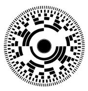
Each separate location can be represented by a binary number, determined by the sequence of light transmission or blockage as you progress inward to the center.
