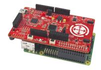
The kit features a set of on-board sensors, including an Ambient Light Sensor, a 3-Axis Accelerometer and a Temperature Sensor. The kit also has an on-board RGB LED, a user-button and a 1-Mbit Cypress F-RAM device.
