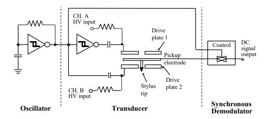
Figure 1. Simplified schematic diagram of the electrostatic transducer used in the new profiler. The stylus force is controlled by the application of DC voltages to the drive plates, and displacement of the stylus is determined from the voltage between the pickup electrode and the lower drive plate.
