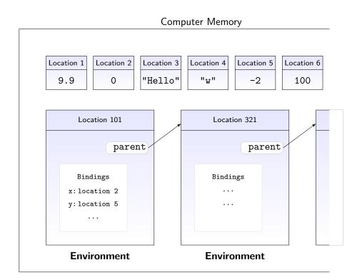
Figure 2.1: A schematic representation of an environment and its enclosing environment.
