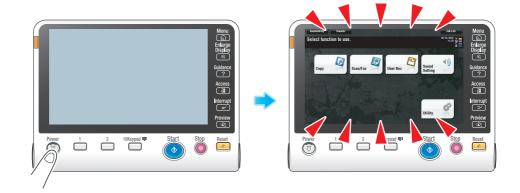
• Check to see that the **Main Power Switch** and the **Power** key are turned ON.
