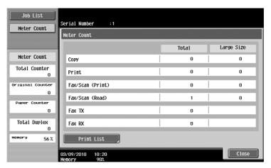
Total: Displays the total page count of Copy, Print, Fax/Scan (Print), Fax/Scan (Read), Fax TX, and Fax RX. Large Size: Displays the large-sized page count of Copy, Print, Fax/Scan (Print), Fax/Scan (Read), Fax TX, and Fax RX.
