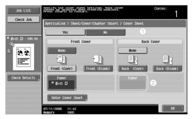
If the optional post inserter has been installed, [Outer Cover Sheet] appears.
