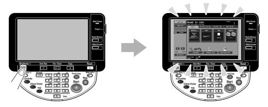
Touch the touch panel. There is no problem if the touch panel lights up. When the machine is in Power Save mode, touching the touch panel or pressing a key in the control panel cancels Power Save mode.
