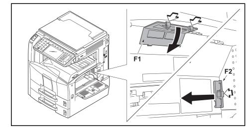
**18** Open the Multi Purpose Tray and remove the filters F1 and F2.
