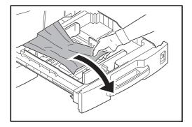
3 Lift duplex unit and remove any paper.
