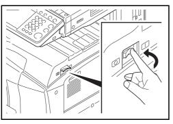
Open the main power switch cover and turn the main power switch on.
