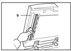
If black streaks or dirt appears in copies when using the optional document processor, clean the slit glass with the supplied cleaning cloth. The message *Clean the slit glass*. may be displayed if the slit glass requires cleaning.
