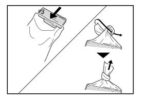
**11** Put the waste toner box in the supplied plastic bag for disposal and securely tie the mouth of the bag.
