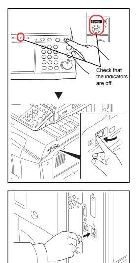
2 Connect the LAN cable to the network interface located on right side of the body.
