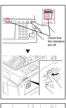
When the machine is powered up, first press the Power key on the operation panel. Check that the Power indicator and the memory indicator are off. After this, turn off the main power switch.
