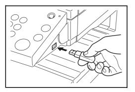
1 Plug the USB memory into the USB memory slot (A1).
