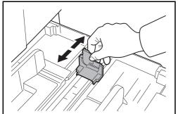
2 Using the paper length guide, move the plate to fit the paper.
