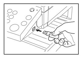
1 Plug the USB memory into the USB memory slot (A1).
