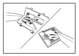
**19** Remove dust from the filters using a vacuum cleaner or dry cloth.
