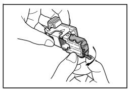
6 Insert the staple holder into the slot of the staple unit again. When fully inserted, the staple holder locks with a clicking sound.
