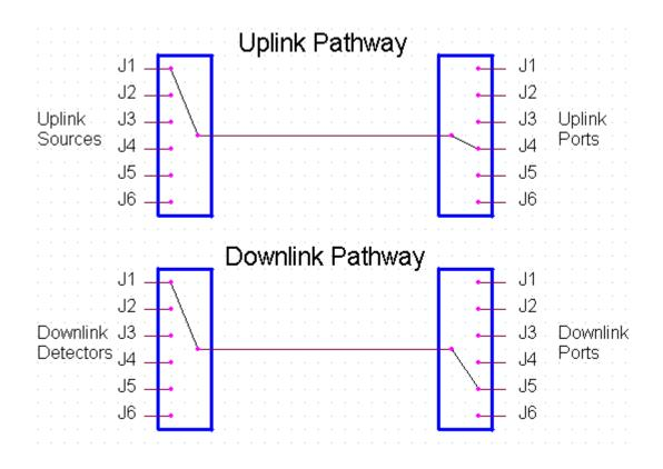
Figure 11.3-2: Switch Position Block Diagram
