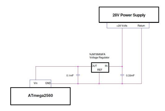
Figure 8-1: 9 Volt Power Regulation Circuit
