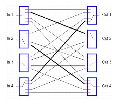
Figure 1.2-1: 4x4 Switch Matrix Function View
