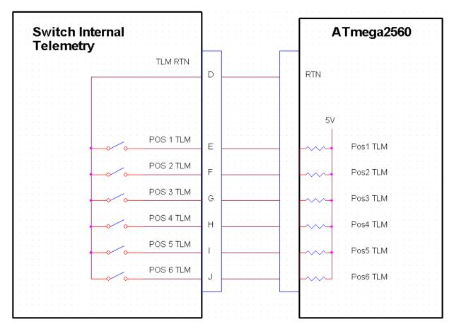
Figure 6.1-1: Switch Telemetry Diagram
