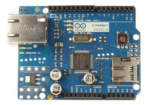
Figure 4.3-1: Arduino Ethernet Shield
