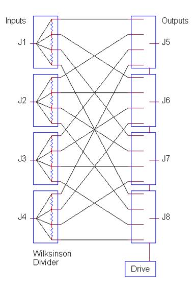
Figure 1.2-5: Full Access (Non-Blocking) Design
