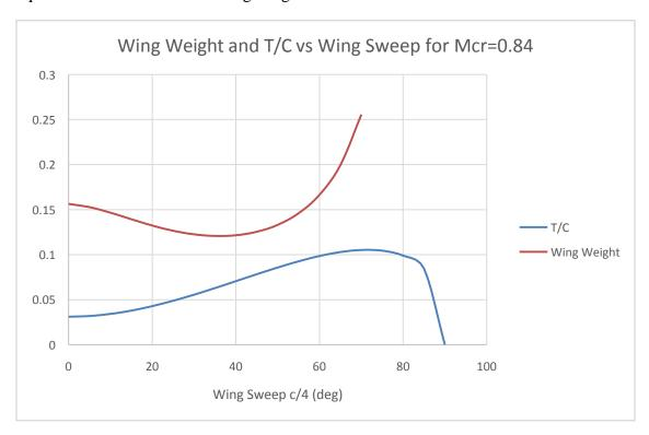
Figure 2.6a: Wing Weight and Thickness Ratio for Different Wing Sweep
