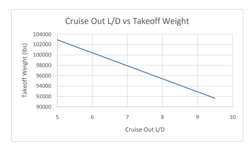
Figure 2.3f: Cruise-Out L/D vs. Weight Takeoff
