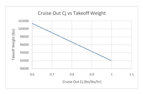
Figure 2.3g: Cruise Out Specific Fuel Consumption vs. Weight Takeoff
