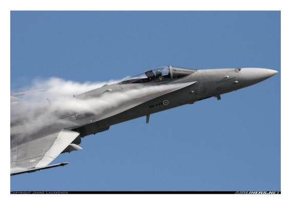
Figure 2.3: Vortex Generated by LERX on a F/A-18.
