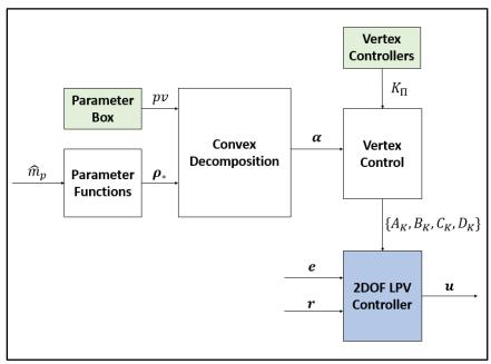
Figure 6.4 – High-level representation of controller matrices generation
