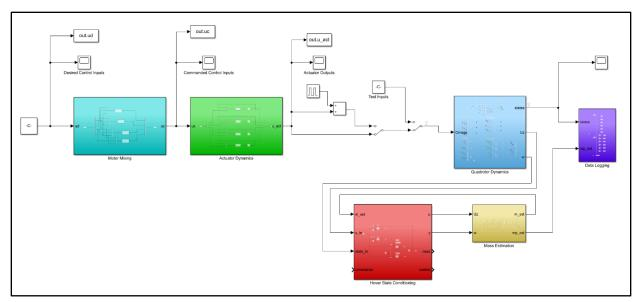
Figure 4.5 – Simulink system with mass estimation and hover state conditioning subsystems
