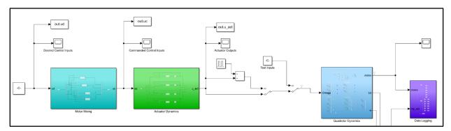
Figure 2.5 – Simulink model of actuator and quadrotor dynamics
