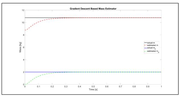
Figure 8.6 – Nonlinear simulation of mass estimation
