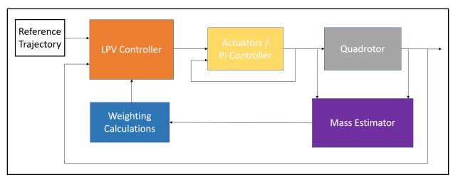
Figure 1.6 - Proposed two-degrees-of-freedom control structure
