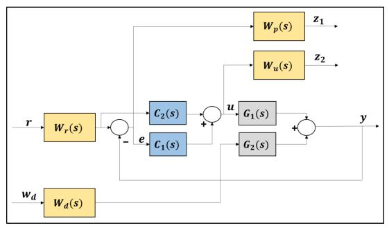
Figure 6.1 – Expanded 2DOF control structure
