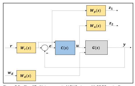
Figure 5.2 – Simplified interconnected LPV System with 2DOF controller
