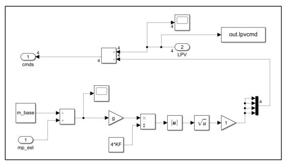
Figure B.10 – Control conditioning for propeller based LPV controller
