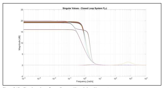
Figure 8.13 – Singular values of propeller speed based closed loop system
