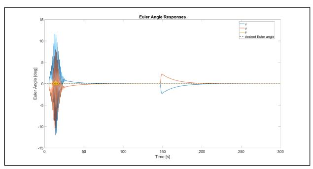
Figure 8.9 – Nonlinear simulation of Euler angle responses
