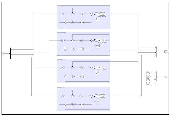
Figure B.6 – 2DOF PI Actuator Controller
