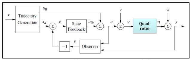
Figure 1.4 - Two-degrees-of-freedom quadrotor control structure [10]
