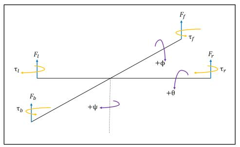
Figure 2.2 – Schematic for rotor and rigid body rotations
