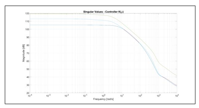
Figure 8.12 – Singular values plot of propeller speed based LPV controller
