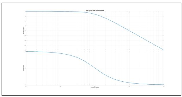
Figure 8.16 – Bode plot for reference signal with  $au_{ref}=0.1$
