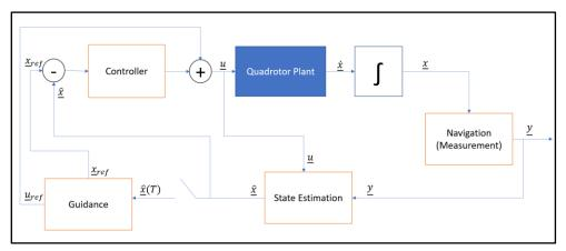
Figure 9.2 – General guidance, navigation, and control system
