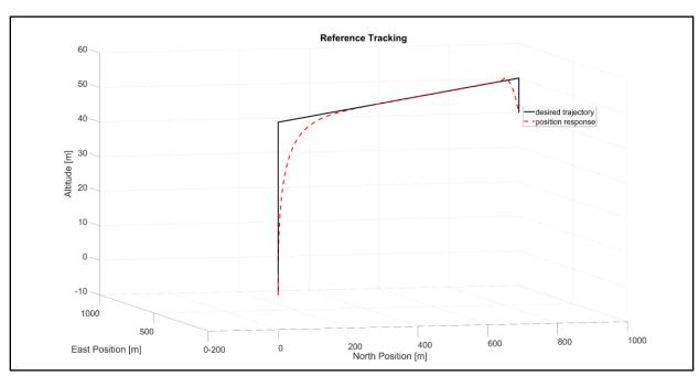
Figure 8.18 – Trajectory tracking against nonlinear system with actuator dynamics
