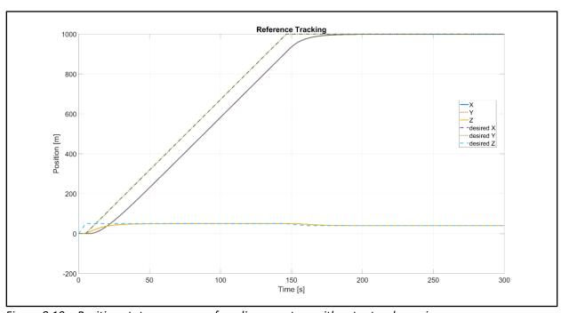
Figure 8.19 – Position state responses of nonlinear system with actuator dynamics
