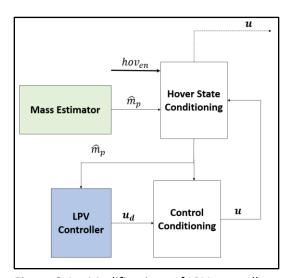
Figure 8.1 - Modifications of LPV controller
