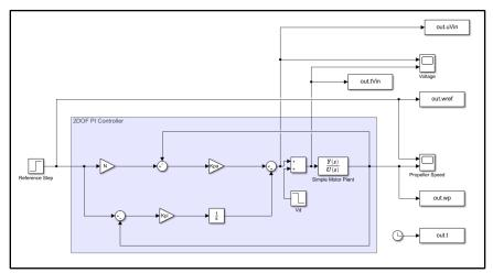
Figure 7.3 – Simulink setup for PI controller
