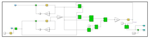
Figure 4.1 – Simulink implementation of mass estimator based on gradient descent law
