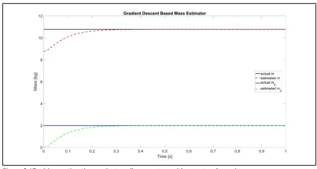
Figure 8.17 – Mass estimation against nonlinear system with actuator dynamics
