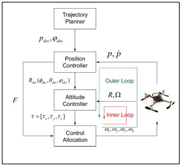
Figure 1.3 - Successive loop closure for a quadrotor  $\overline{[10]}$
