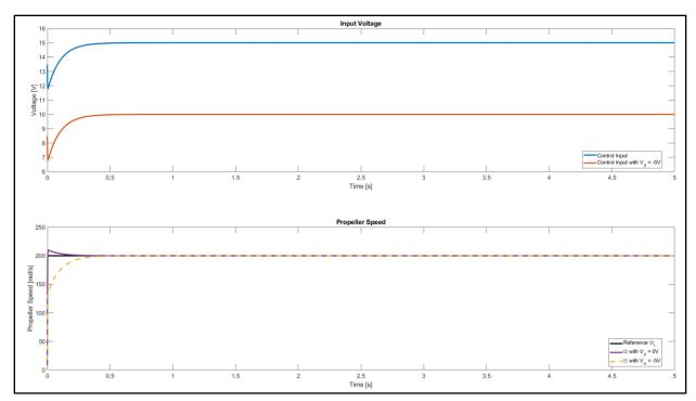
Figure 7.4 – Propeller speed response subject to voltage change
