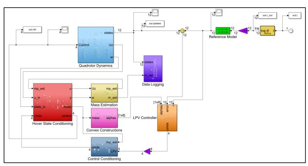
Figure 8.4 – Nonlinear simulation setup with desired forces and torques as inputs
