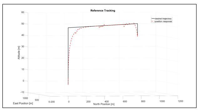
Figure 8.24 – Trajectory tracking against nonlinear system with disturbances
