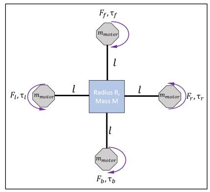
Figure 2.4 – Quadrotor top-view schematic for design parameters
