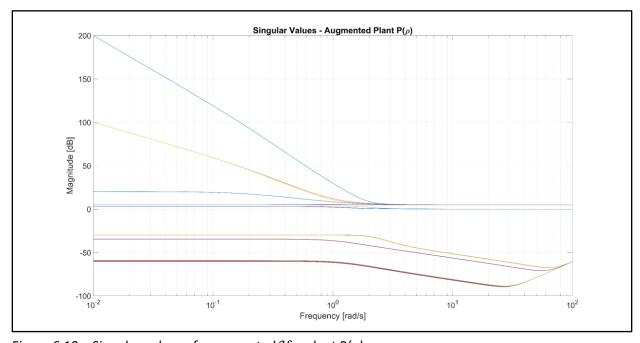
Figure 6.10 – Singular values of augemented  $\mathcal{H}_{\infty}$  plant P(p)
