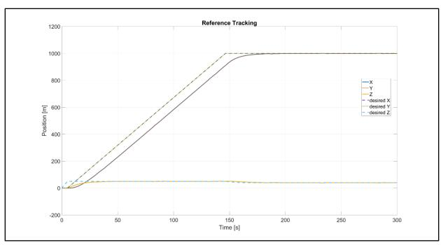
Figure 8.25 - Position state responses of nonlinear system with disturbances
