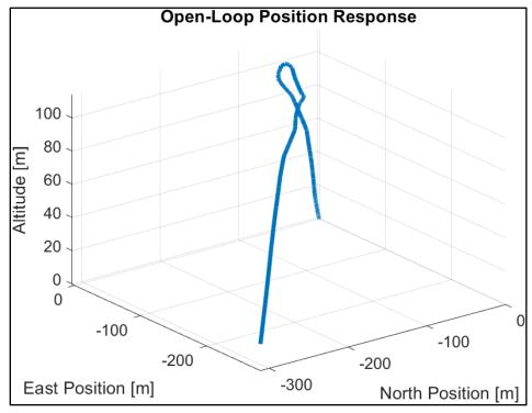
Figure 2.7 – Open-loop response of inertial positions
