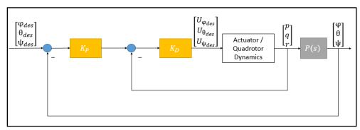
Figure C.1 – PD control structure for attitude control
