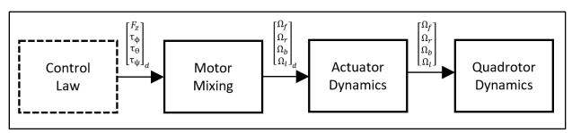
Figure 2.3 – Motor Mixing and Actuator Dynamics
