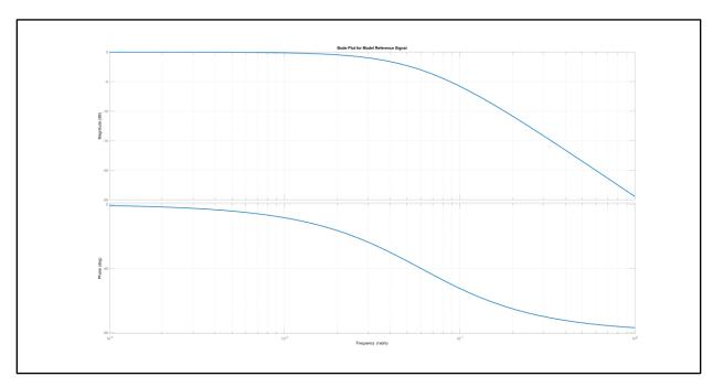
Figure 8.2 – Bode plot of model reference signal  $\textit{G}_{r}(\textit{s})$  with  $\tau_{ref} = 0.06$
