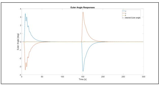
Figure 8.21 – Euler angle state responses of nonlinear system with actuator dynamics
