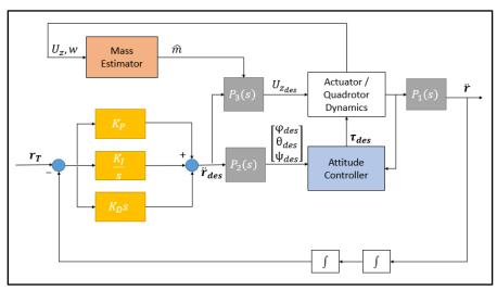
Figure C.2 – Position control integrated into the control system
