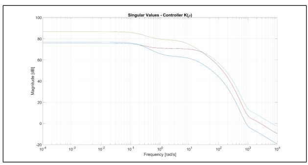
Figure 6.11 – Singular values of polytopic LPV controller  $K(\rho)$
