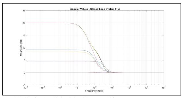
Figure 6.12 – Singular values of polytopic closed-loop system  $F(\rho)$
