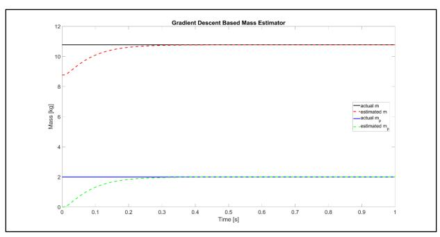
Figure 8.23 – Mass estimation against nonlinear system with disturbances
