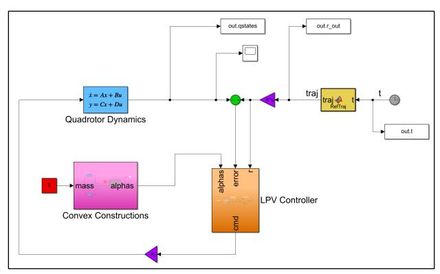
Figure 6.19 – Simulink setup for linear simulation
