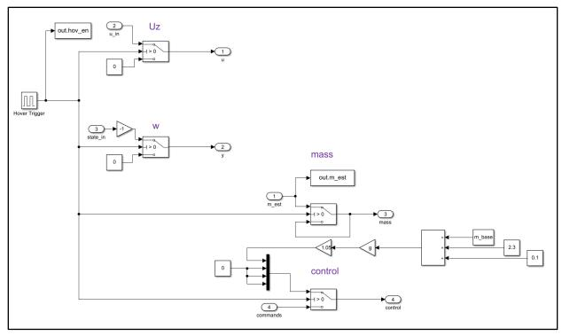
Figure 4.4 – Simulink implementation of hover state conditioning
