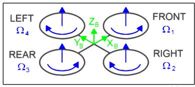
Figure 1.1 - Propeller speeds in hovering condition [1]
