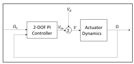
Figure 7.1 – Simplified diagram for propeller speed regulation
