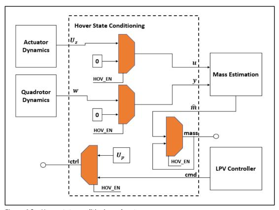
Figure 4.3 – Hover state conditioning subsystem
