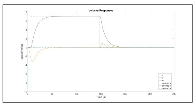
Figure 8.20 – Velocity state responses of nonlinear system with actuator dynamics
