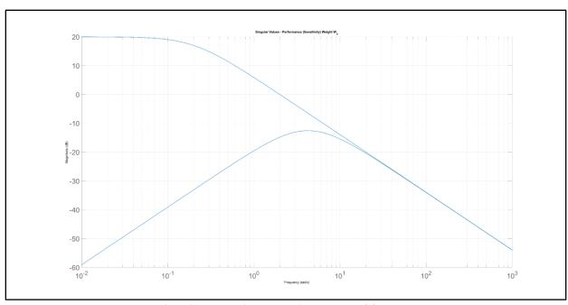
Figure 6.2 – Singular values of performance (sensitivity) weight  $W_p(s)$
