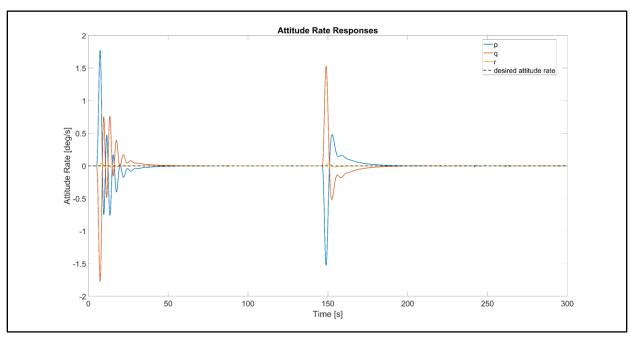
Figure 8.22 – Attitude rate state responses of nonlinear system with actuator dynamics
