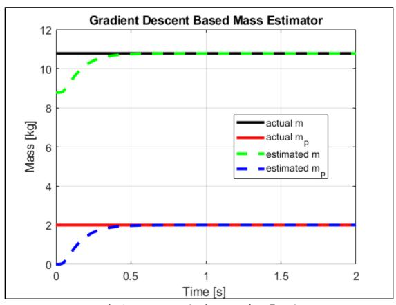
Figure 4.6 – Estimation of unknown mass with information from  $\textit{F}_{\textit{z}}$  and w
