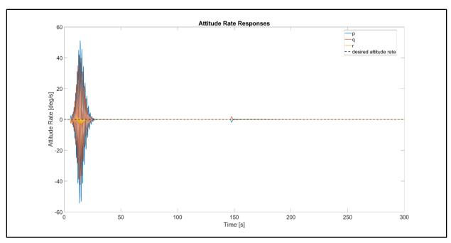
Figure 8.10 – Nonlinear simulation of attitude rate responses
