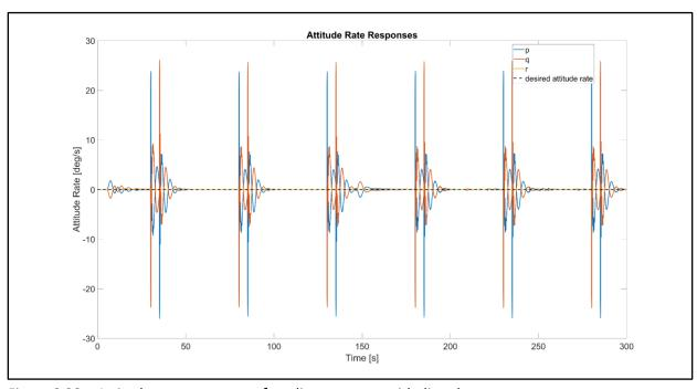
Figure 8.28 – Attitude rate responses of nonlinear system with disturbances
