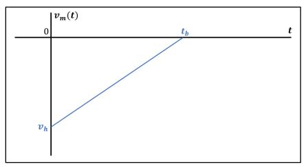
Figure 6.17 – Linear decrease of velocity to 0 at landing position
