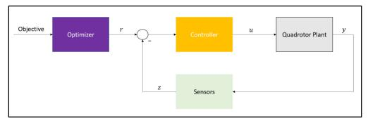
Figure 9.1 – Optimizer and controller
