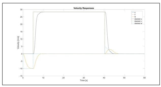
Figure 6.21 – Velocity tracking for linear simulation
