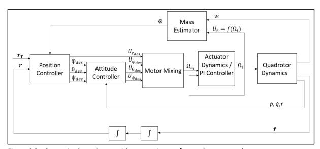
Figure C.3 – Successive loop closure with mass estimator for quadrotor control
