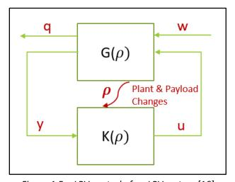
Figure 1.5 - LPV control of an LPV system [16]
