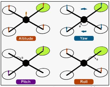
Figure 1.2 - Basic quadrotor control actions [3]
