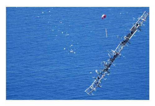
Figure 9: Helios HP03 Complete Structural Failure [3]
