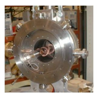
Figure 17 Actual Helicon antenna Source: Baity, 2003
