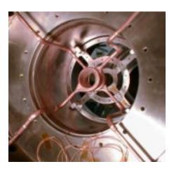
Figure 19 Actual ICRH antenna Source: Bering, 2006
