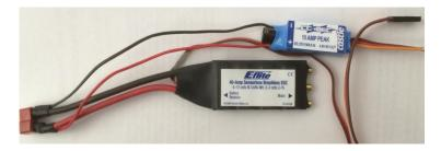
Figure 6. ESC and BEC
