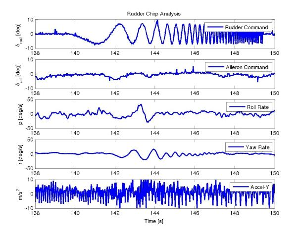
Figure 11. Rudder automated chirp analysis
