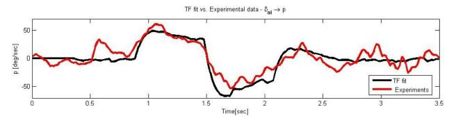
Figure 15. Roll Rate Response to Doublet Command of 7 degrees of aileron de ection
