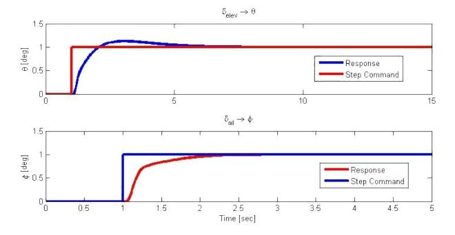
Figure 10. Closed loop response for 1<sup>o</sup> step input.
