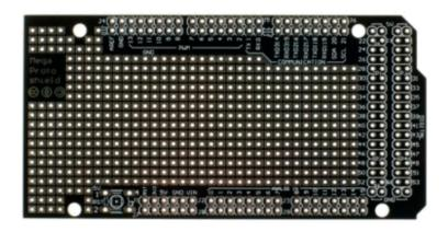
Figure 2. Arduino Mega Shield Top View
