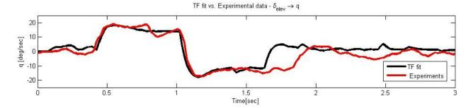
Figure 14. Pitch Rate Response to Doublet Command of 7 degrees of elevator de ection
