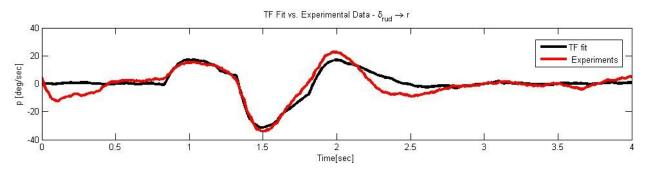
Figure 13. Yaw Rate Response to Doublet Command of 7 degrees of rudder de ection
