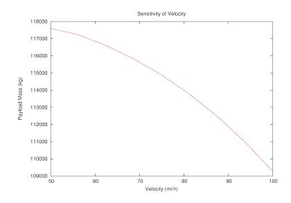
Figure 4.5: Sensitivity of payload mass to nominal velocity (mi/h)
