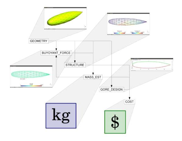
Figure 4.1: Design structure matrix and representative outputs for the example model
