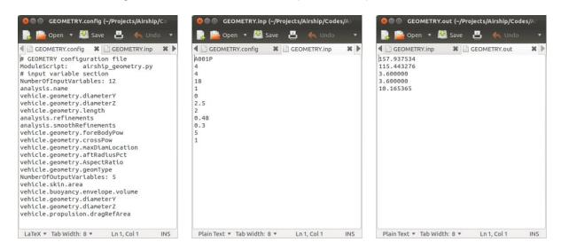
Figure 3.8: Comparison of a con guration le and its respective module input and output les. Note that the order of the variables in the con guration le corresponds to the order in the input and output les.
