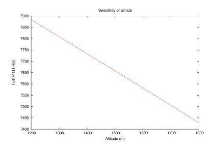
Figure 4.8: Sensitivity of propulsion fuel mass to altitude
