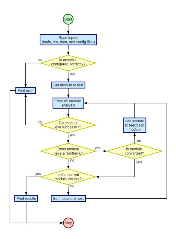
Figure 3.1: Flow diagram of the analysis function in COEUS
