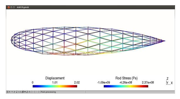
Figure 4.4: Structural module plot illustrating displacement and beam stress
