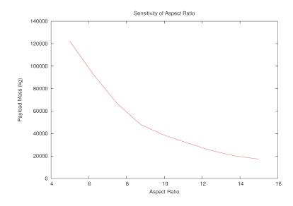
Figure 4.7: Sensitivity of payload mass to vehicle aspect ratio
