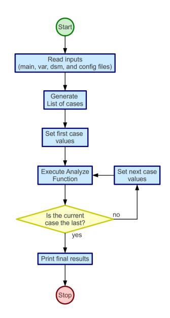
Figure 3.2: Flow diagram of the main function in COEUS
