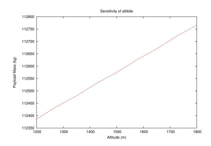
Figure 4.6: Sensitivity of payload mass to nominal altitude (m)
