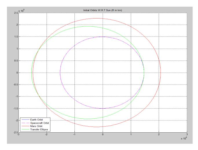
Figure 5.1: Graphical representation of Hohmann Transfer maneuver
