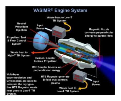
Figure 1.1: Schematic Diagram of a VASIMR SYSTEM [4]
