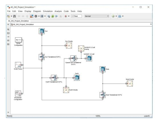
Figure 3.1: Simulink model for generating 3-D astrodynamics simulation
