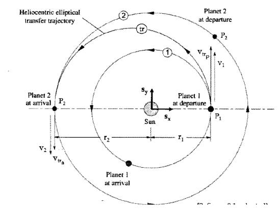
Figure 2.1: Depiction of Ideal Hohmann Transfer Scenario between two circular orbits
