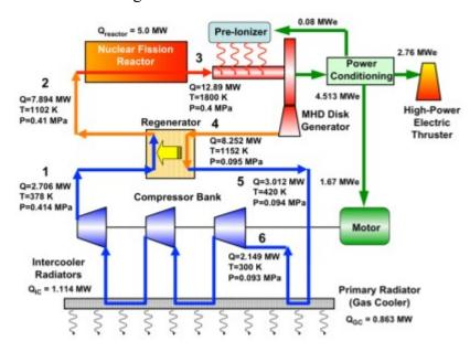
Figure 1.3: General architecture of a nuclear, multi-MW MHD-VASIMR sys. [5]
