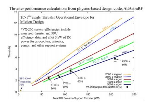
Figure 1.2: System Performance Curves for Argon and Krypton [2]
