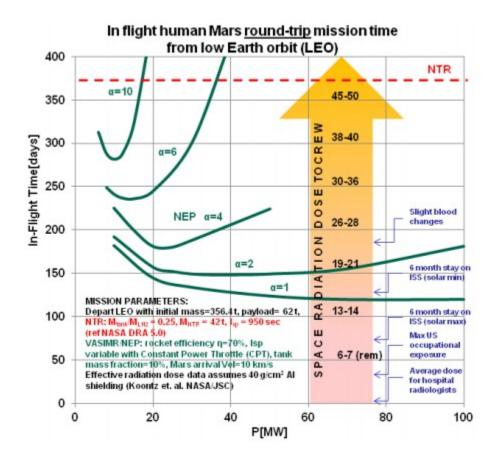
Figure 1.4: Radiation exposure against in-flight duration vs power required for VASIMR human Mars Mission [5]
