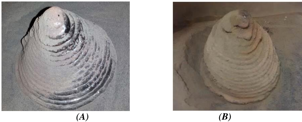
Figure 6.1: 3D-printed regolith simulant, (A) hollow cone and (B) hollow dome structure [20].
