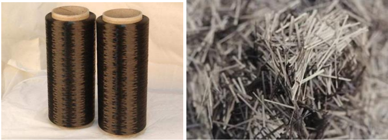
Figure 3.2: Macro- and microscopic views of basalt fiber [28].
