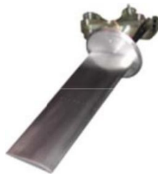
Figure 3.3 - Clark Y-14 Airfoil ( AEROLAB, 2007)
