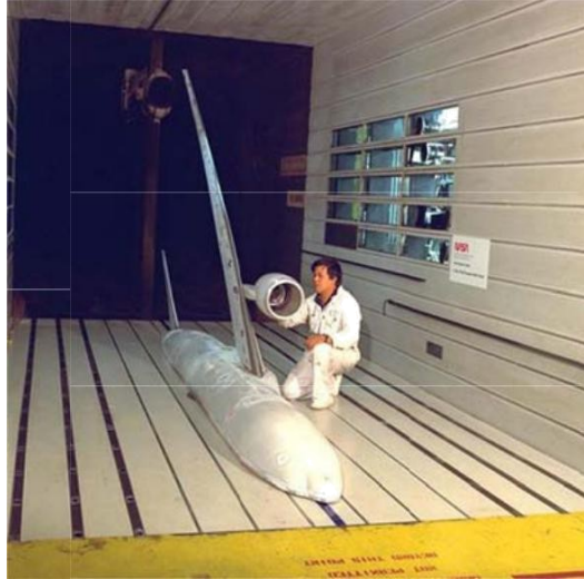
Figure 1.4b - Example of model mounted on test section wall. (NASA, 2005)
